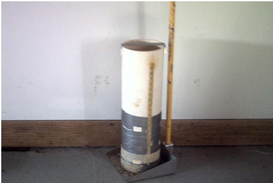
Figure 1. Leaf Pack Core Sampler
