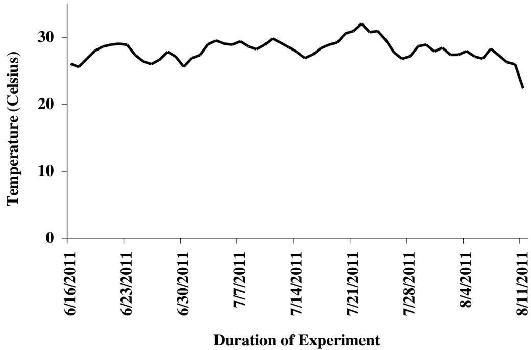
**Figure 19** Daily temperature reading of laboratory conditions: An EasyLog EL-USB-2 - Humidity, Temperature and Dew Point Data Logger (with LCD) was the instrument that recorded laboratory conditions throughout the duration of this experiment. It was set to automatically take a reading every five minutes. This information was then loaded into an Excel data sheet for analysis and interpretation. An average was calculated for each day.
