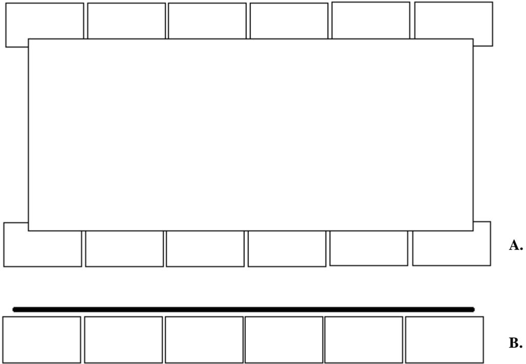
**Figure 3** Experimental platform: The experimental platform consisted of five pieces: a frame, a platform, plastic sheeting, felt strips and twelve plastic containers. This structure held the spiderling pairs prior to and during an experiment; the experimental and temporary experimental chambers were placed on this structure (A. overhead view, B. side view).
