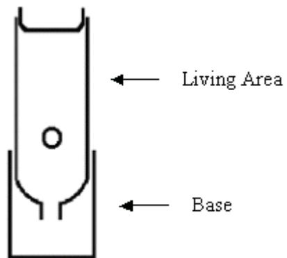
**Figure 1** Spider holding chamber: These chambers were made from colorless 3-liter soda bottles and consisted of two sections, a base and living area. This device was used to house adult female spiders. In total, 40 of these chambers were constructed for this experiment.
